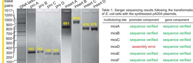
Figure 10. 2% (w/v) analytical agarose gel electrophoresis; successful transformation of *E. coli* cells with pAD04 plasmids containing the synthesized promoter (pro) and insert sequences.
