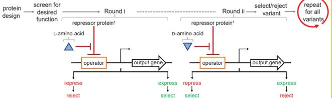
Figure 1. Engineering proteins that recognize or produce metabolites with enantiomeric specificity requires that protein variant functions be screened using multiple rounds of the protein engineering workflow. For example, engineering a repressor that selectively recognizes an L-amino acid requires screening the same candidate protein to ensure no interaction with the D-amino acid enantiomer. This renders the conventional protein engineering workflow intractable and prone to failure.
